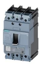
circuit breaker 3VA5 UL frame 125 breaking capacity class M 35kA @ 480 V 3-pole, line protection TM230, FTAM, In=90A overload protection Ir=90A fixed short-circuit protection Ii=5...10 x In UL489 SB (naval), 50 deg. cel. cable connection on both sides
