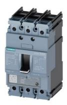
circuit breaker 3VA5 UL frame 125 breaking capacity class M 35kA @ 480 V 3-pole, line protection TM230, FTAM, In=90A overload protection Ir=90A fixed short-circuit protection Ii=5...10 x In cable connection on both sides
