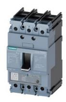
circuit breaker 3VA5 UL frame 125 breaking capacity class S 25kA @ 480 V 3-pole, line protection TM230, FTAM, In=90A overload protection Ir=90A fixed short-circuit protection Ii=5...10 x In cable connection on both sides
