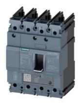
circuit breaker 3VA5 UL frame 125 breaking capacity class H 65kA @ 480V 4-pole, line protection TM230, FTAM, In=80A overload protection Ir=80A fixed short-circuit protection Ii=5...10 x In N conductor unprotected without connection
