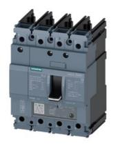
circuit breaker 3VA5 UL frame 125 breaking capacity class M 35kA @ 480 V 4-pole, line protection TM230, FTAM, In=60A overload protection Ir=60A fixed short-circuit protection Ii=5...10 x In N conductor unprotected without connection
