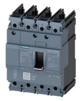
circuit breaker 3VA5 UL frame 125 breaking capacity class H 65kA @ 480V 4-pole, line protection TM210, FTFM, In=50A overload protection Ir=50A fixed short-circuit protection li=10 x In N conductor unprotected without connection
