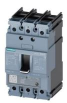
circuit breaker 3VA5 UL frame 125 breaking capacity class H 65kA @ 480 V 3-pole, line protection TM230, FTAM, In=50A overload protection Ir=50A fixed short-circuit protection Ii=5...10 x In cable connection on both sides
