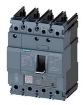
circuit breaker 3VA5 UL frame 125 breaking capacity class S 25kA @ 480V 4-pole, line protection TM240, ATAM, In=50A overload protection Ir=40A...50A short-circuit protection Ii=5...10 x In N conductor unprotected without connection
