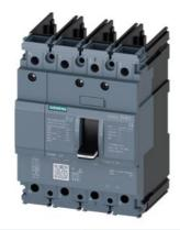
circuit breaker 3VA5 UL frame 125 breaking capacity class S 25kA @ 480V 4-pole, line protection TM210, FTFM, In=50A overload protection Ir=50A fixed short-circuit protection Ii=10 x In N conductor unprotected without connection
