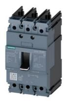
circuit breaker 3VA5 UL frame 125 breaking capacity class S 25kA @ 480V 3-pole, line protection TM210, FTFM, In=50A overload protection Ir=50A fixed short-circuit protection Ii=10 x In without connection
