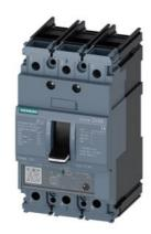
circuit breaker 3VA5 UL frame 125 breaking capacity class S 25kA @ 480 V 3-pole, line protection TM230, FTAM, In=50A overload protection Ir=50A fixed short-circuit protection Ii=5...10 x In nut keeper kit on both sides
