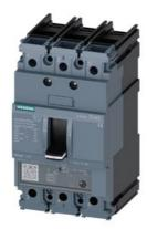
circuit breaker 3VA5 UL frame 125 breaking capacity class H 65kA @ 480 V 3-pole, line protection TM230, FTAM, In=45A overload protection Ir=45A fixed short-circuit protection Ii=5...10 x In UL489 SB (naval), 50 deg. cel. nut keeper kit on both sides
