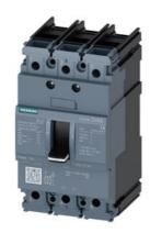
circuit breaker 3VA5 UL frame 125 breaking capacity class S 25kA @ 480 V 3-pole, line protection TM210, FTFM, In=45A overload protection Ir=45A fixed short-circuit protection Ii=10 x In nut keeper kit on both sides
