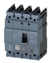
circuit breaker 3VA5 UL frame 125 breaking capacity class M 35kA @ 480 V 4-pole, line protection TM230, FTAM, In=40A overload protection Ir=40A fixed short-circuit protection Ii=5...10 x In N conductor unprotected without connection
