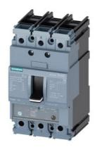
circuit breaker 3VA5 UL frame 125 breaking capacity class S 25kA @ 480 V 3-pole, line protection TM240, ATAM, In=40A overload protection Ir=32A ...40A short-circuit protection Ii=5...10 x In cable connection on both sides
