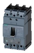
circuit breaker 3VA5 UL frame 125 breaking capacity class S 25kA @ 480 V 3-pole, line protection TM240, ATAM, In=40A overload protection Ir=32A ...40A short-circuit protection Ii=5...10 x In nut keeper kit on both sides
