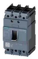
circuit breaker 3VA5 UL frame 125 breaking capacity class S 25kA @ 480 V 3-pole, line protection TM210, FTFM, In=40A overload protection Ir=40A fixed short-circuit protection Ii=10 x In UL489 SB (naval), 50 deg. cel. nut keeper kit on both sides
