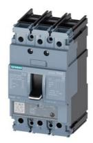
circuit breaker 3VA5 UL frame 125 breaking capacity class S 25kA @ 480 V 3-pole, line protection TM230, FTAM, In=40A overload protection Ir=40A fixed short-circuit protection Ii=5...10 x In cable connection on both sides
