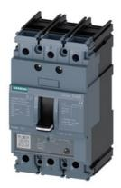
circuit breaker 3VA5 UL frame 125 breaking capacity class S 25kA @ 480 V 3-pole, line protection TM230, FTAM, In=40A overload protection Ir=40A fixed short-circuit protection Ii=5...10 x In nut keeper kit on both sides
