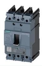
circuit breaker 3VA5 UL frame 125 breaking capacity class S 25kA @ 480V 3-pole, line protection TM230, FTAM, In=40A overload protection Ir=40A fixed short-circuit protection li=5...10 x In UL 489 SB (naval), 50° C without connection
