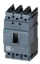
circuit breaker 3VA5 UL frame 125 breaking capacity class H 65kA @ 480V 3-pole, line protection TM210, FTFM, In=35A overload protection Ir=35A fixed short-circuit protection Ii=10 x In UL 489 SB (naval),  $50^\circ$  C without connection
