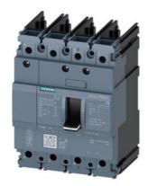
circuit breaker 3VA5 UL frame 125 breaking capacity class S 25kA @ 480V 4-pole, line protection TM210, FTFM, In=35A overload protection Ir=35A fixed short-circuit protection Ii=10 x In N conductor unprotected without connection
