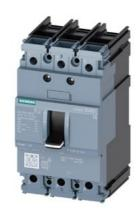
circuit breaker 3VA5 UL frame 125 breaking capacity class S 25kA @ 480 V 3-pole, line protection TM210, FTFM, In=35A overload protection Ir=35A fixed short-circuit protection Ii=10 x In UL489 SB (naval), 50 deg. cel. cable connection on both sides
