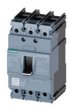
circuit breaker 3VA5 UL frame 125 breaking capacity class S 25kA @ 480 V 3-pole, line protection TM210, FTFM, In=35A overload protection Ir=35A fixed short-circuit protection li=10 x In cable connection on both sides
