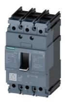
circuit breaker 3VA5 UL frame 125 breaking capacity class S 25kA @ 480 V 3-pole, line protection TM210, FTFM, In=35A overload protection Ir=35A fixed short-circuit protection Ii=10 x In nut keeper kit on both sides
