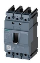
circuit breaker 3VA5 UL frame 125 breaking capacity class S 25kA @ 480V 3-pole, line protection TM210, FTFM, In=35A overload protection Ir=35A fixed short-circuit protection li=10 x In UL 489 SB (naval), 50° C without connection
