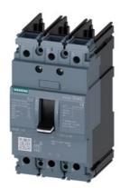
circuit breaker 3VA5 UL frame 125 breaking capacity class S 25kA @ 480V 3-pole, line protection TM210, FTFM, In=35A overload protection Ir=35A fixed short-circuit protection Ii=10 x In without connection
