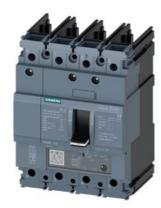
circuit breaker 3VA5 UL frame 125 breaking capacity class S 25kA @ 480V 4-pole, line protection TM230, FTAM, In=35A overload protection Ir=35A fixed short-circuit protection Ii=5...10 x In N conductor unprotected without connection
