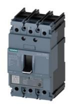
circuit breaker 3VA5 UL frame 125 breaking capacity class S 25kA @ 480 V 3-pole, line protection TM230, FTAM, In=35A overload protection Ir=35A fixed short-circuit protection Ii=5...10 x In UL489 SB (naval), 50 deg. cel. nut keeper kit on both sides
