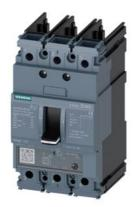
circuit breaker 3VA5 UL frame 125 breaking capacity class S 25kA @ 480V 3-pole, line protection TM230, FTAM, In=35A overload protection Ir=35A fixed short-circuit protection Ii=5...10 x In without connection
