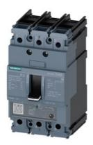
circuit breaker 3VA5 UL frame 125 breaking capacity class M 35kA @ 480 V 3-pole, line protection TM230, FTAM, In=30A overload protection Ir=30A fixed short-circuit protection Ii=5...10 x In nut keeper kit on both sides
