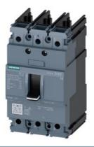
circuit breaker 3VA5 UL frame 125 breaking capacity class S 25kA @ 480V 3-pole, line protection TM210, FTFM, In=30A overload protection Ir=30A fixed short-circuit protection Ii=10 x In UL 489 SB (naval),  $50^\circ$  C without connection
