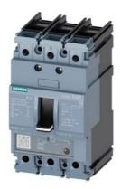
circuit breaker 3VA5 UL frame 125 breaking capacity class S 25kA @ 480 V 3-pole, line protection TM230, FTAM, In=30A overload protection Ir=30A fixed short-circuit protection Ii=5...10 x In cable connection on both sides
