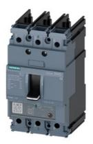
circuit breaker 3VA5 UL frame 125 breaking capacity class S 25kA @ 480V 3-pole, line protection TM230, FTAM, In=30A overload protection Ir=30A fixed short-circuit protection Ii=5...10 x In UL 489 SB (naval), 50° C without connection
