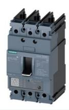
circuit breaker 3VA5 UL frame 125 3-pole, starter protection TM120M, AM, In=30A without overload protection short-circuit protection li=3...7 x In without connection
