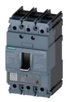
circuit breaker 3VA5 UL frame 125 breaking capacity class H 65kA @ 480 V 3-pole, line protection TM230, FTAM, In=25A overload protection Ir=25A fixed short-circuit protection Ii=6...12 x In nut keeper kit on both sides
