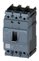
circuit breaker 3VA5 UL frame 125 breaking capacity class S 25kA @ 480 V 3-pole, line protection TM210, FTFM, In=25A overload protection Ir=25A fixed short-circuit protection Ii=12 x In UL489 SB (naval), 50 deg. cel. nut keeper kit on both sides
