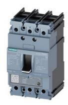
circuit breaker 3VA5 UL frame 125 breaking capacity class S 25kA @ 480 V 3-pole, line protection TM230, FTAM, In=25A overload protection Ir=25A fixed short-circuit protection Ii=6...12 x In cable connection on both sides
