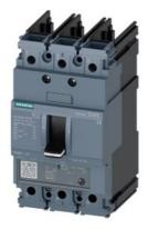
circuit breaker 3VA5 UL frame 125 breaking capacity class S 25kA @ 480V 3-pole, line protection TM230, FTAM, In=25A overload protection Ir=25A fixed short-circuit protection Ii=6...12 x In UL 489 SB (naval), 50° C without connection
