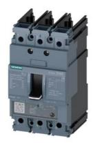
circuit breaker 3VA5 UL frame 125 breaking capacity class S 25kA @ 480V 3-pole, line protection TM230, FTAM, In=25A overload protection Ir=25A fixed short-circuit protection Ii=6...12 x In without connection
