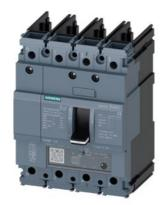
circuit breaker 3VA5 UL frame 125 breaking capacity class H 65kA @ 480V 4-pole, line protection TM230, FTAM, In=20A overload protection Ir=20A fixed short-circuit protection Ii=7.5...15 x In N conductor unprotected without connection
