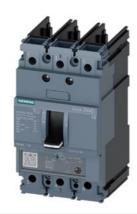
circuit breaker 3VA5 UL frame 125 breaking capacity class M 35kA @ 480 V 3-pole, line protection TM230, FTAM, In=20A overload protection Ir=20A fixed short-circuit protection Ii=7.5...15 x In UL 489 SB (naval), 50° C without connection
