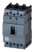
circuit breaker 3VA5 UL frame 125 breaking capacity class H 65kA @ 480 V 3-pole, line protection TM210, FTFM, In=125A overload protection Ir=125A fixed short-circuit protection Ii=10 x In nut keeper kit on both sides
