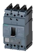
circuit breaker 3VA5 UL frame 125 breaking capacity class H 65kA @ 480V 3-pole, line protection TM230, FTAM, In=125A overload protection Ir=125A fixed short-circuit protection Ii=5...10 x In without connection
