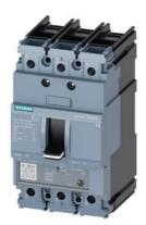
circuit breaker 3VA5 UL frame 125 breaking capacity class M 35kA @ 480 V 3-pole, line protection TM230, FTAM, In=125A overload protection Ir=125A fixed short-circuit protection Ii=5...10 x In UL489 SB (naval), 50 deg. cel. cable connection on both sides
