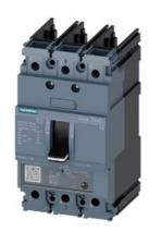
circuit breaker 3VA5 UL frame 125 breaking capacity class M 35kA @ 480V 3-pole, line protection TM230, FTAM, In=125A overload protection Ir=125A fixed short-circuit protection Ii=5...10 x In UL 489 SB (naval), 50° C without connection
