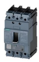
circuit breaker 3VA5 UL frame 125 breaking capacity class H 65kA @ 480 V 3-pole, line protection TM230, FTAM, In=110A overload protection Ir=110A fixed short-circuit protection Ii=5...10 x In nut keeper kit on both sides
