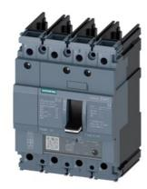
circuit breaker 3VA5 UL frame 125 breaking capacity class S 25kA @ 480V 4-pole, line protection TM230, FTAM, In=110A overload protection Ir=110A fixed short-circuit protection Ii=5...10 x In N conductor unprotected without connection
