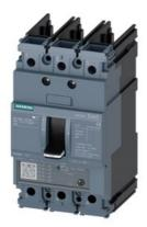
circuit breaker 3VA5 UL frame 125 3-pole, starter protection TM120M, AM, In=110A without overload protection short-circuit protection Ii=3...7 x In without connection
