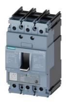
circuit breaker 3VA5 UL frame 125 breaking capacity class M 35kA @ 480 V 3-pole, line protection TM230, FTAM, In=100A overload protection Ir=100A fixed short-circuit protection Ii=5...10 x In cable connection on both sides
